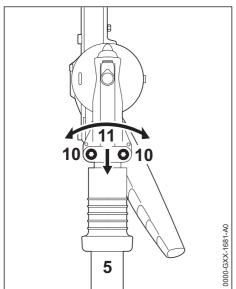
► Loosen the clamp screws (10).
